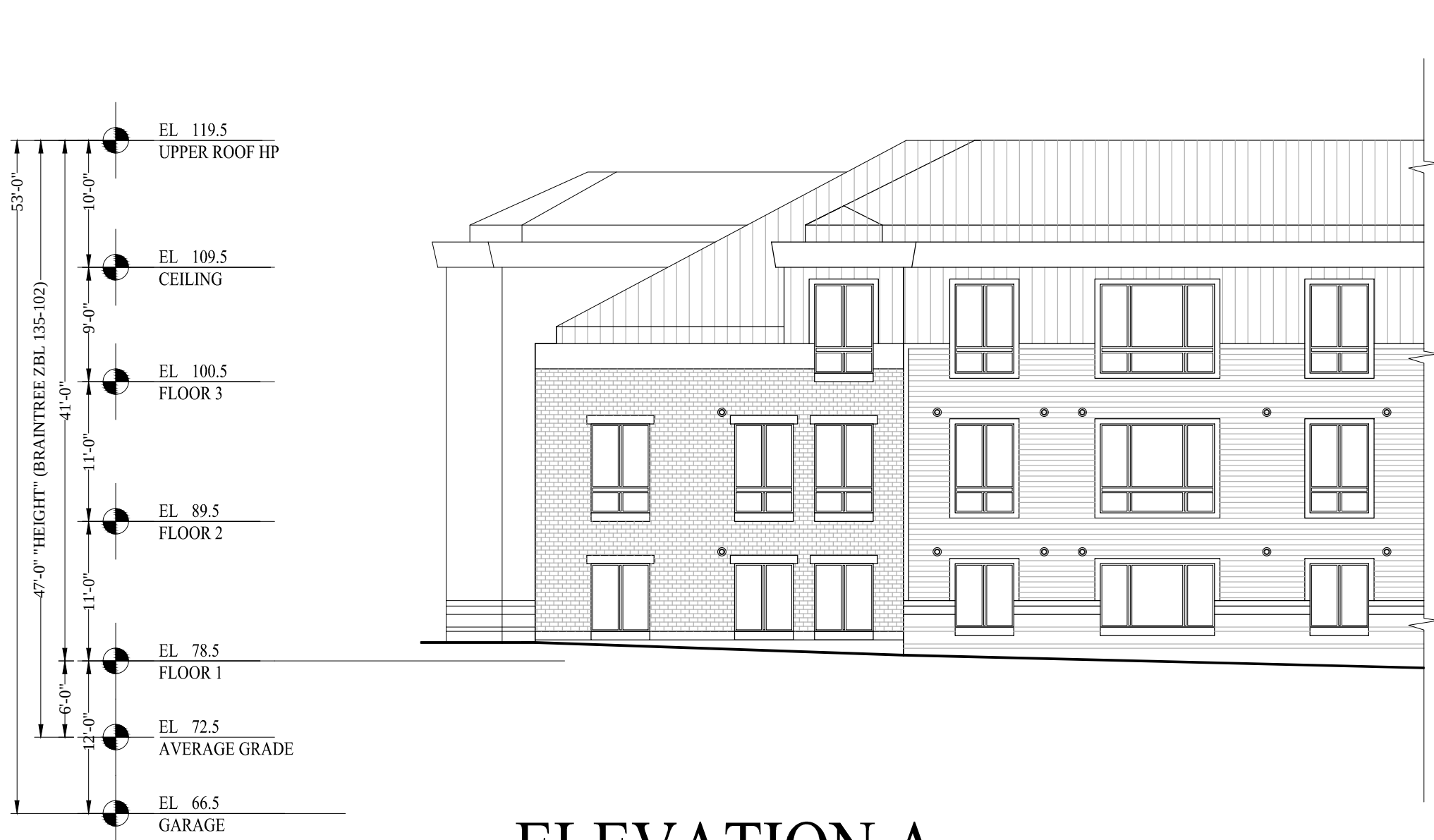
ELEVATION A (NORTH-NORTHEAST-EAST - MAIN ENTRANCE COURT)
